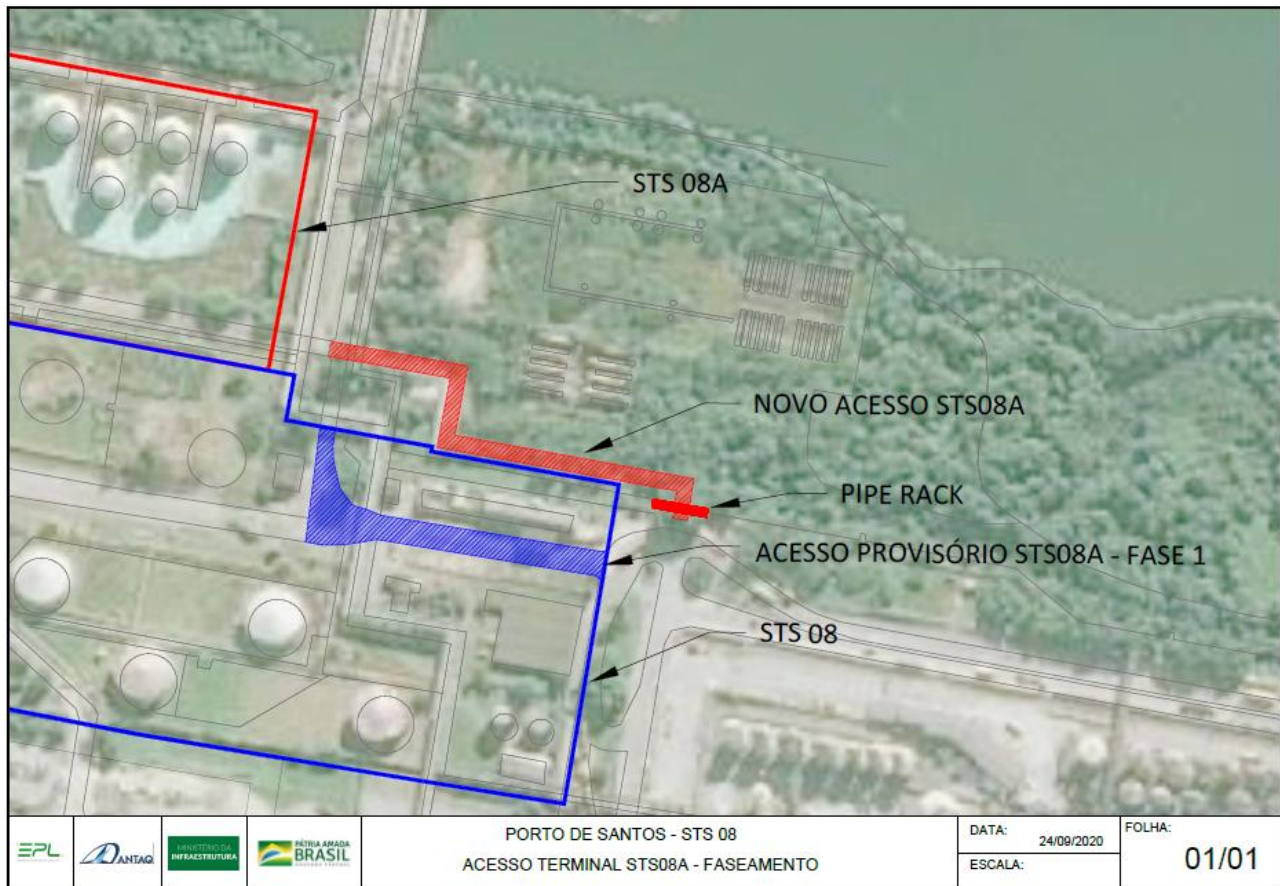
Figure 5: Phasing - Terminal Access Source: EPL
